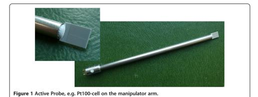
The procedure stores the value of power necessary to maintain the temperature balance level at set-point temperature without energy influx and controls the temperature balance level by analysing the value and the changing rate of the probe temperature. Also it calculates the difference between the power currently needed and the power needed without energy influx from plasma. It displays directly if measurement starts the incoming energy influx at the probe in mW.
