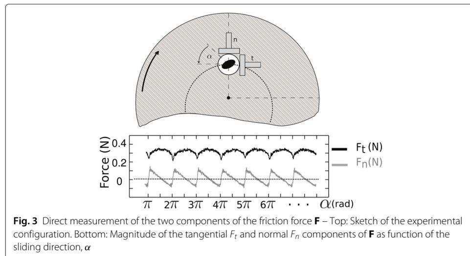
**Fig. 3** Direct measurement of the two components of the friction force  $\mathbf{F}$  – Top: Sketch of the experimental configuration. Bottom: Magnitude of the tangential  $F_t$  and normal  $F_n$  components of  $\mathbf{F}$  as function of the sliding direction,  $\alpha$
