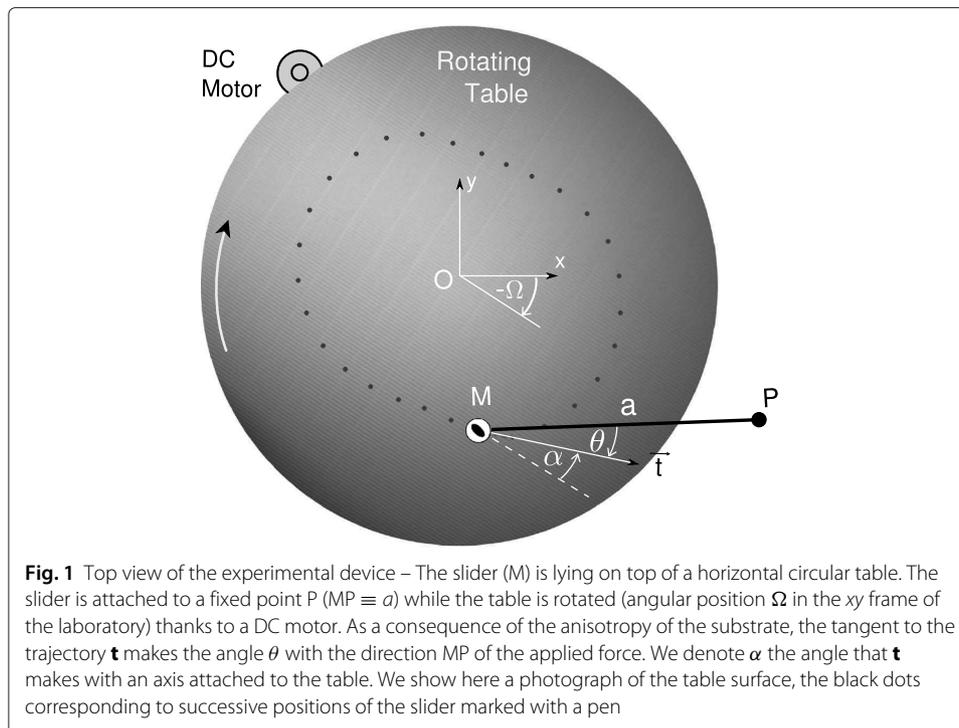
(Agilent, E3641A). The resulting rotation speed,  $\omega$ , ranges from 1–14 rpm. The angular position of the table  $\Omega = \omega t$  is measured, with an accuracy of 1 deg, thanks to a coupled diode-photodiode system which locates black and white stripes drawn on the lower surface of the table.
