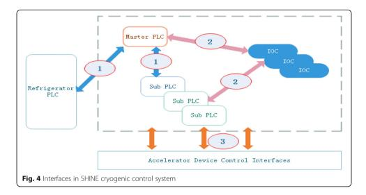
refrigerator PLC and other sub PLCs. Master to refrigerator is read only with a shared memory table to avoid impact to it; Master to sub is read/write through register address with PLC configuration technology.
