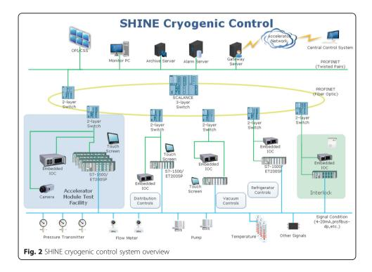
In the core of the control system, powerful Linux servers host the operational files and run other application software based on JAVA or script languages.
