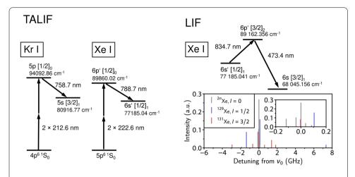
**Figure 3** Excitation schemes used in the present work. Left: TALIF schemes in neutral krypton and neutral xenon. Right: LIF scheme in neutral xenon (top), spectral positions (line broadening excluded) of the hyperfine structure lines (bottom)
