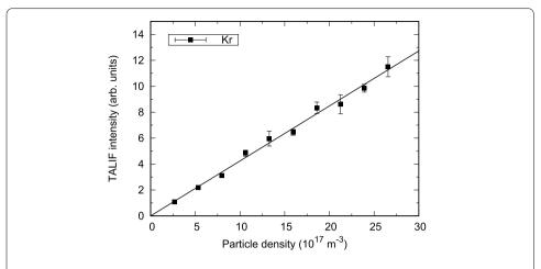
**Figure 6** TALIF signal measured for krypton background densities in the vacuum facility, measured during cold gas flow operation at a distance appropriately aside the thruster axis
