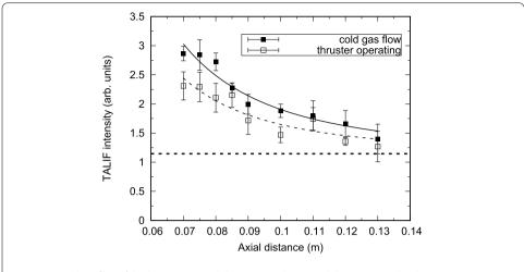
**Figure 7** Axial profiles of the krypton neutral densities on the central thruster axis. The distances are given to the accelerator grid on the center axis
