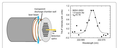
**Figure 10** Left: Directions of excitation and fluorescence detection in a TALIF approach inside the discharge chamber of an ion source. Right: TALIF profile in the discharge chamber for the indicated operation condition
