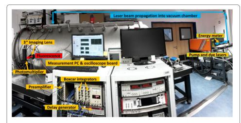
**Figure 2** TALIF set-up for ion thruster diagnostics as realized in the lab at IOM. Image modified from Eichhorn et al. Paper IEPC-2019-503 [79]
