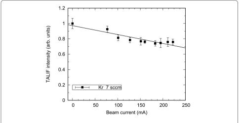
**Figure 9** TALIF signal intensity depending on the beam current at fixed mass flow, as a measure for the mass utilization efficiency
