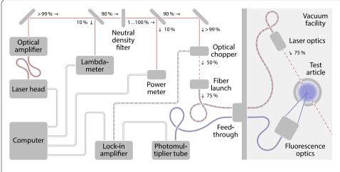
**Figure 4** Schematics of the LIF setup. Optical transmissions or reflectances of each element placed in the laser beam path are denoted, optical fibers are visualized by curved lines
