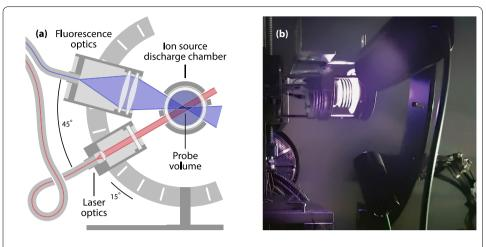
**Figure 5** (a) Schematics of the LIF vacuum optics arrangement (not to scale). The effective viewing angles of the optical probes are restricted due to supporting elements of the ion source; the intermediate angle between laser propagation and detection axis was set to 45 degrees for optimum laser insertion and fluorescence detection. (b) Ion source discharge chamber and the LIF vacuum setup in side view
