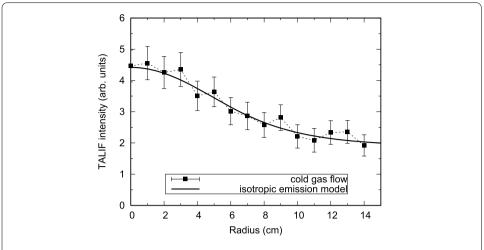
**Figure 8** Radial profile of the krypton density at the axial distance of 8 cm. Adopted from Eichhorn et al. Paper IEPC-2019-503 [79]
