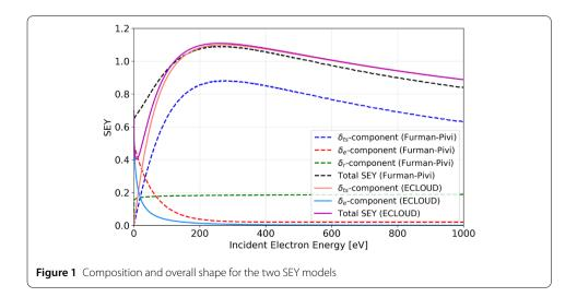
with  $\hat{E}_t \simeq \hat{E}_{ts} = 276.8 \text{ eV}$ ,  $\hat{E}_e = 0 \text{ eV}$ ,  $E_r = 0.041 \text{ eV}$ , for the PEP-II surface pipe sample [17, 26]. The variation of SEY components with respect to incident electron energy for SEY = 1.1 is illustrated in Fig. 1. Even if the total secondary electron yield parameter has the same value, slight differences between the two models are observed, as e.g. the rediffused electron component of the SEY is not included in the ECLOUD model.
