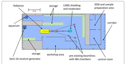
**Figure 1** Floor plan for the Nuclear Applications Laboratory, Lund University, with key features of the layout, and major infrastructure components, labelled. The new CANS, which must compete for space in already busy laboratory environment, is place between the pre-existing IBA beamlines
