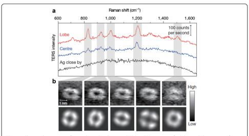
**Fig. 11** Chemical mapping of a single molecule using TERS. **a** TER spectra of a lobe and the centre of an individual  $H_2$ TBPP molecule and the silver substrate (**b**) TERS maps of different Raman modes from an individual  $H_2$ TBPP molecule (top panel) and the corresponding TERS maps simulated with density functional theory (DFT). Reprinted with permission from Macmillan Publishers Ltd: NATURE [7], copyright 2012
