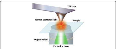
**Fig. 1** Schematic diagram of a TERS set-up. A schematic diagram illustrating the principle of AFM-TERS in transmission mode. The LSP resonance at the tip-apex between the tip-LSPs and laser-photons enhances and confines the EM field resulting in the enhancement of Raman signal from the analyte molecules in the immediate vicinity of the tip-apex
