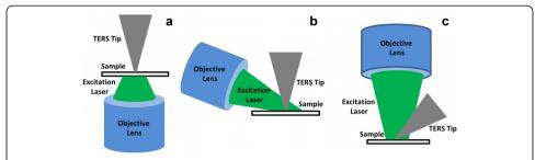
**Fig. 3** Schematic diagrams of most commonly used TERS configurations. **a** Bottom illumination set-up. **b** Side illumination set-up. **c** Top illumination set-up
