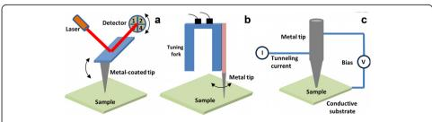
**Fig. 5** Schematic diagrams of SPM feedback mechanisms used in TERS. **a** AFM feedback mechanism. **b** Shear-force feedback mechanism. **c** STM feedback mechanism
