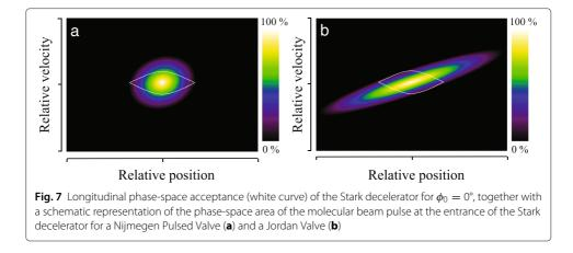
performance of a JV as a source for Stark decelerators is best described using an *effective* opening time  $\tau$  that is much smaller than the actual opening duration of the valve.
