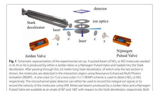
beams are collimated by a skimmer (s) and a collimator (c). These beams allow for scattering experiments, but in this study they are used to characterize the velocity distribution of the conventional beams
