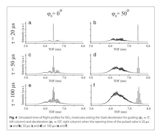
*b*),  $\tau = 50 \ \mu s$  (panels *c* and *d*), and  $\tau = 100 \ \mu s$  (panels *e* and *f*). These are representative values for  $\tau$  for an NPV, JV, and GV, respectively.
