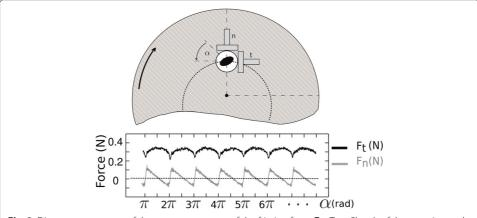
**Fig. 3** Direct measurement of the two components of the friction force  $\mathbf{F}$  – Top: Sketch of the experimental configuration. Bottom: Magnitude of the tangential  $F_t$  and normal  $F_n$  components of  $\mathbf{F}$  as function of the sliding direction,  $\alpha$
