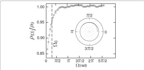
**Fig. 2** Radius  $\rho$  vs. angular position  $\Omega$  – We observe that the asymptotic trajectory is reached after a typical rotation of about  $\Omega_c=a/\rho_0\simeq 0.7$  rad in our experimental conditions. Inset: trajectory of the slider in the table frame (continuous line) [isotropic friction, a=12.3 cm and R=22.1 cm]
