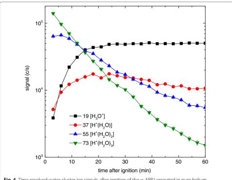
Fig. 4 Time-resolved water cluster ion signals after ignition of the  $\mu$ -APPJ operated in pure helium connected via a tube made from stainless steel
