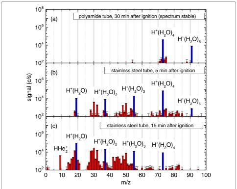
**Fig. 3** Effect of Type of feed gas connection ((a) polyamide tube; (b) stainless steel 5 min After ignition; (c) stainless steel 15 min after ignition) on mass spectra obtained from the analysis of the  $\mu$ -APPJ operated in a controlled atmosphere, no admixture of reactive gases, 2 mm distance to orifice
