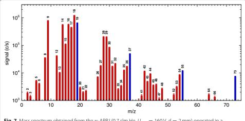
**Fig. 7** Mass spectrum obtained from the  $\mu$ -APPJ (0.7 slm He,  $U_{rms}=160\,\text{V}$ ,  $d=2\,\text{mm}$ ) operated in a controlled atmosphere. Possible ion assignments are presented in Table 1
