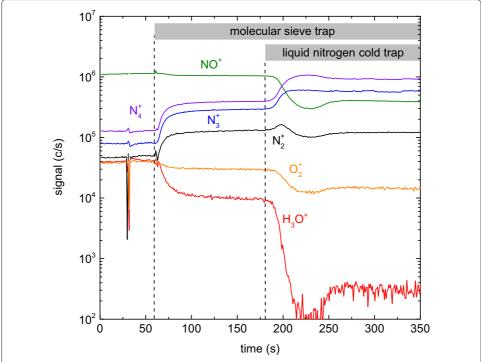
**Fig. 5** Time-resolved measurement showing the significant effect of two purification methods (molecular sieve trap at  $t=60\,\mathrm{s}$  and liquid nitrogen trap at  $t=180\,\mathrm{s}$ ) applied to the feed gas line of the  $\mu$ -APPJ operated at a gas flow rate of 1.4 slm He and an admixture of 0.25 %  $N_2$ . The admixture of nitrogen is mandatory for stable operating conditions
