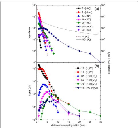
**Fig. 8** Selected ion signals from  $\mu$ -APPJ (0.7 slm He,  $U_{rms} = 160 \text{ V}$ , d = 2 mm) in dependence on the distance to the sampling orifice orifice. The assignments in square brackets are corresponding to the most likely ion. For clarity the ions are separated into to groups summarizing (**a**) non-water and (**b**) water-containing ions. The dashed lines show the expected trends for N<sup>+</sup> and NO<sup>+</sup> based on reactions (4) and (10), respectively
