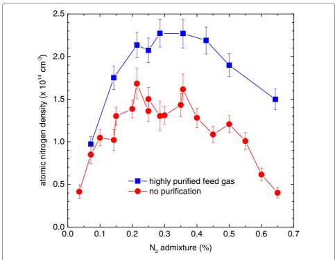
Fig. 6 Effect of purification by molecular sieve trap and liquid nitrogen trap on the density of atomic nitrogen in a  $\mu$ -APPJ operated in 1.4 slm He with an variable admixture of  $N_2$  measured by molecular beam mass spectrometry (MBMS) [34]
