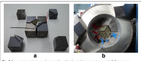
**Fig. 2** The experimental setup: **a** the assembly within the eight tungsten inner anvils. **b** The pressure module with outer anvils surrounding the cube of inner anvils
