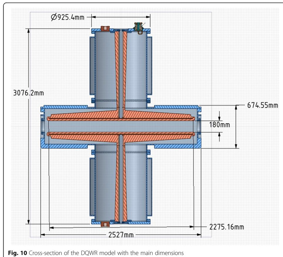
**Fig. 10** Cross-section of the DQWR model with the main dimensions
