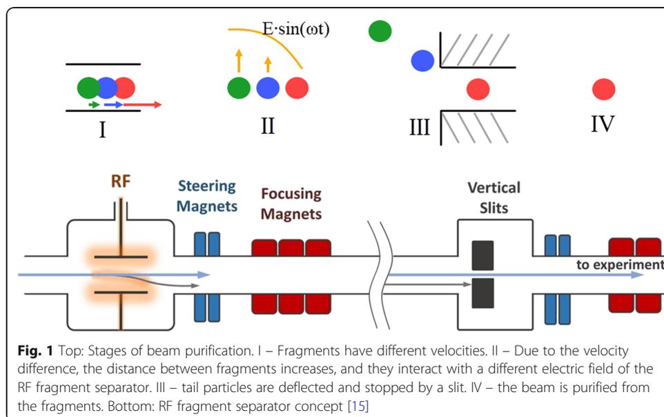
**Fig. 1** Top: Stages of beam purification. I – Fragments have different velocities. II – Due to the velocity difference, the distance between fragments increases, and they interact with a different electric field of the RF fragment separator. III – tail particles are deflected and stopped by a slit. IV – the beam is purified from the fragments. Bottom: RF fragment separator concept [15]
