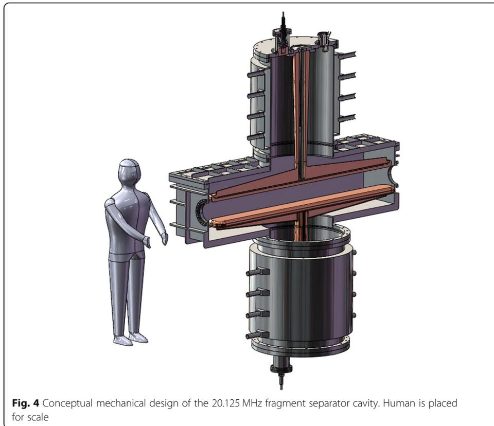
from the bottom to beamline should not exceed 1.5 m, the cavity should operate at 20.125 MHz, the aperture size must be 18 cm, and the voltage between electrodes – 300 kV. Three main classes of resonators were considered: H-resonator, split coaxial resonator and TEM-class resonator.
