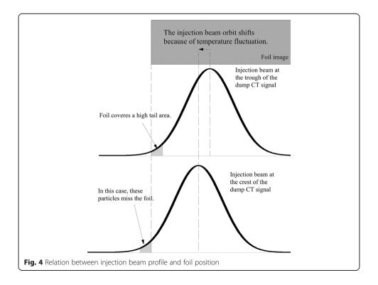
the injection beam orbit. Consequently, when the injection beam is in the inner position, the foil can cover a relatively large area of the beam profile. In contrast, if the beam injects in the outer position, more particles in the tail of the profile would miss the foil and fail in the charge exchange.
