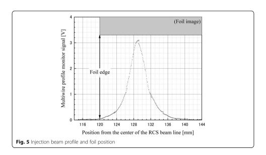
relation between the measured profile data and foil position. The interval between each measurement point is 0.03 mm.
